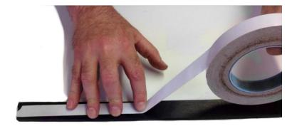
For use as a economical temporary fixing to hold solid rubber, cork or foam gasket strip in position when assembling. Simply peel from roll, place directly on rubber strip and rub down, pull off silicone paper and place gasket in position. In the case of 'self apply' we recommend adhesive tape to be narrower than rubber gasket, example 15mm or 19mm wide to suit 25mm wide rubber strip.
